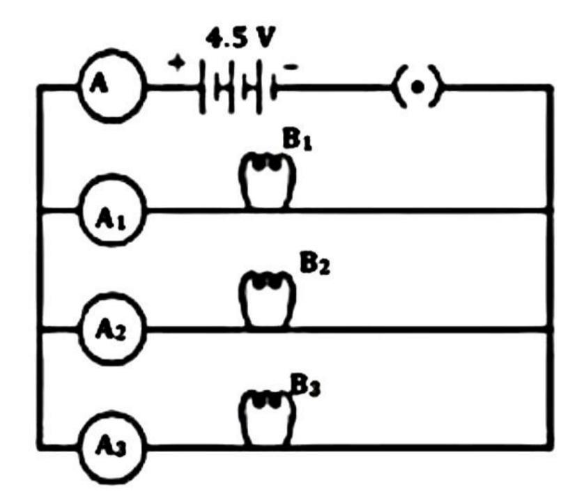
Study the above circuit diagram in which the three identical bulbs B<sub>1</sub>, B<sub>2</sub> and B<sub>3</sub> are connected in parallel with a battery of 4.5 V.
